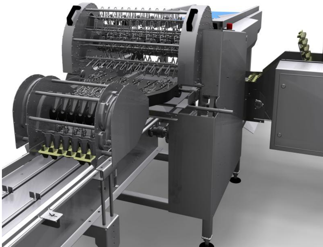
Continuous drop system places the eggs in various trays used worldwide. Removable parts enable external cleaning.
