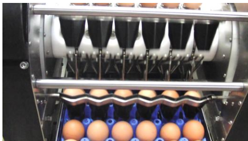
Continuous drop system places the eggs in various trays used worldwide. Removable parts enable external cleaning.
